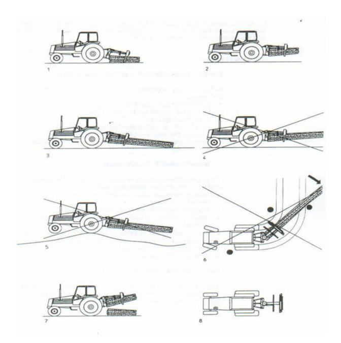
For skidding or pulling a trailer with a 2WD tractor the rule of thumb is to add 10 lb. front-end weights for every horsepower of tractor engine power. Thus on a 40 HP tractor one adds 40 x 10=400 lbs. of front end weights. This assumes "average" conditions and tractors without tire chains. The use of tire chains will increase the traction on inclines, where tires without chains will spin. One must therefore compensate for the increased traction by adding weights in order to
